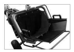
7. Install the intake extension chute and intake extension bar
