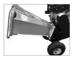
3. Fit the intake hopper Fit the intake hopper and secure the bolts.
